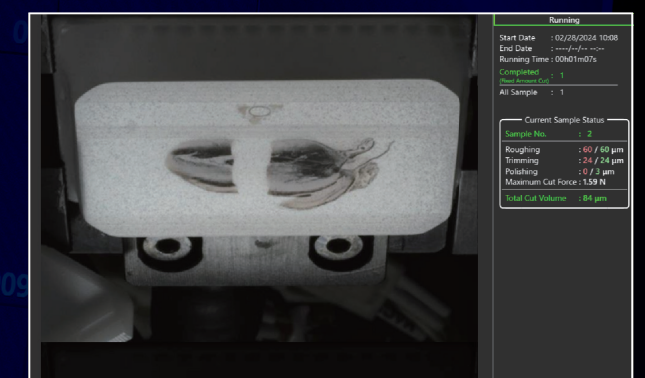
Detailed imaging and logging of each processed block
