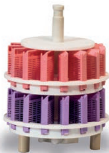
Standard - 30 cassettes For specimens 30x25x5 mm
