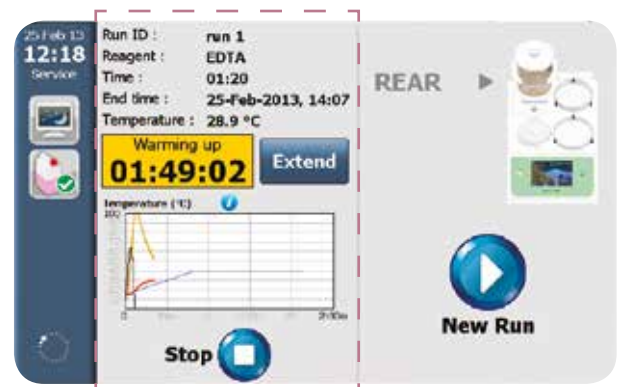
2 - Running a decalcification protocol with temperature curve
