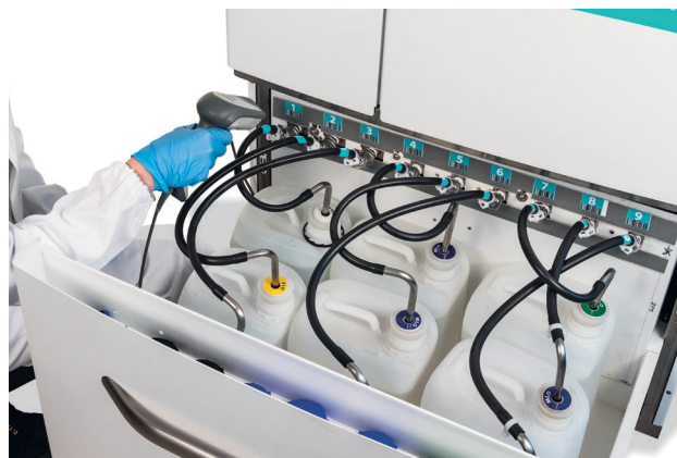
Step 2: reagent loading position scanning
