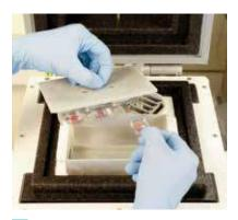
4 Position each cryomold in the slide-in holder.
