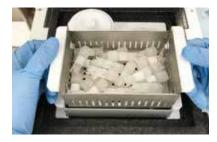
7 Up to 25 cryovials can be simultaneously frozen.
