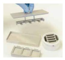
1 The cryomold kit (optional) allows to carry out standardized flash freezing.
