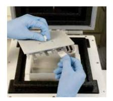
7 Slide the cryomolds from the holder.
