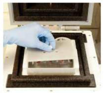
5 Place the slide-in holder on top of the tank. The fluid inside the set level tank freezes only the mold without contaminating the specimen.
